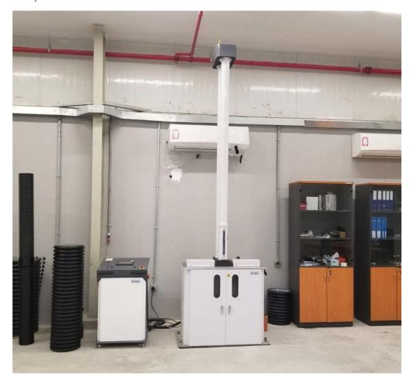
The impact test is tested in accordance with EN 744. The purpose of this test is to determine if the pipe cracks when impacted by a given weight at a 2 meter height. The test is deemed to have passed if there are no visible cracks in the pipe.
