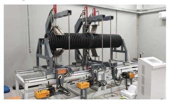
The joint tightness test is a test which measures the tightness of the EPDM rubber gasket at a vacuum pressure. If no leak occurs, then the test is said to have passed.
