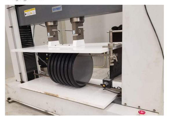
The ring stiffness test is used to determine the pipe's resistance to external forces. A 3% diametric deflection of the internal diameter is applied to the pipe and the stiffness can be calculated in accordance with ISO 9969.
